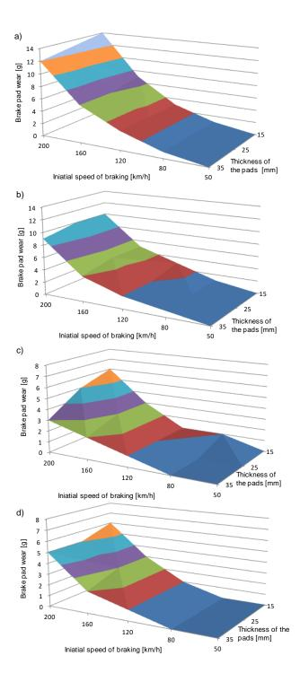
Fig. 5. Mass wear of the pads at: a) N = 40 kN,  $M_h = 6.7 t$ , b) N = = 28 kN,  $M_h = 6.7 t$ , c) N = 26 kN,  $M_h = 4.7 t$ , b) N = 16 kN,  $M_h = 4.7 t$
