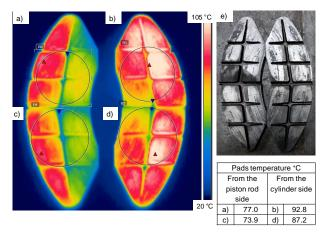
Fig. 6. Temperature distribution on the brake pads, a) upper left pad, b) upper right pad, c) lower left pad, d) lower right pad, e) View of the set of brake pads after braking from the speed of 120 km/h
