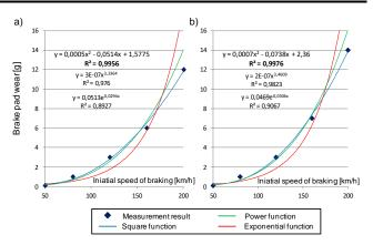
Fig. 3. The relationship of brake pad wear as a function of initial speed at N = 40 kN and  $M_h = 6.7$  t, braking with: a) new 35 mm brake pads, b) 15 mm brake pads
