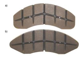
Fig. 2. Friction pads used during the tests: a) type 175, b) type 200, view from the side of contact with the disc
