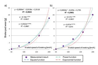
Fig. 4. The relationship of brake pad wear as a function of initial speed at N = 28 kN and  $M_h = 6.7$  t, braking with: a) new 35 mm brake pads, b) 15 mm brake pads
