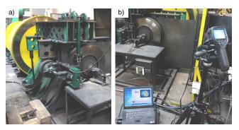
Fig. 1. Stand for testing a railway disc brake: a) view of the working part with rotating masses, b) view of the tested brake disc with thermal imaging measurement
